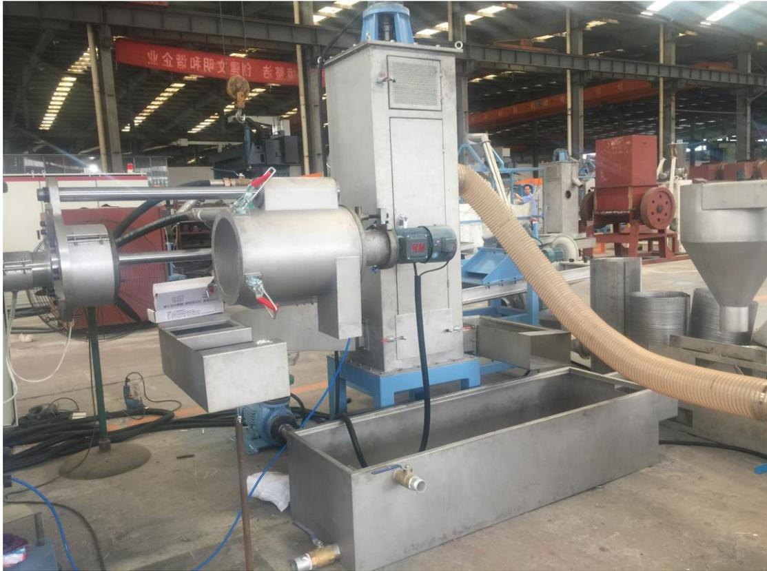
Crushed film recycling pellet machine is used for crushed film pelletizing, feeding method is Screw force feeder
